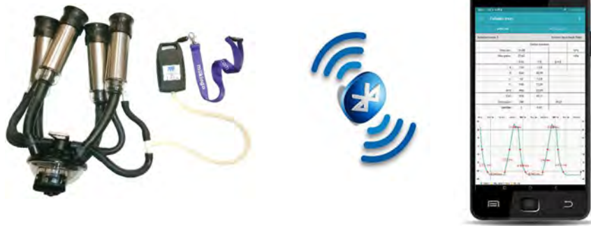
Bluetooth link among the elements of the DPT system
